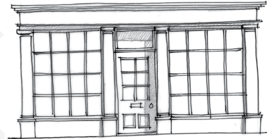
Figure 2. Georgian Shopfront Colonnade filled with glazing and stallriser
