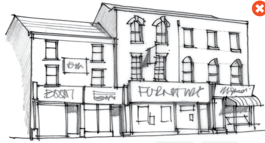
Figure 8. Fascias designed disregarding individual buildings, features and street rhythm
